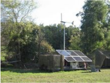
Desalination System TSS 100 including wind generator set up on a military camp in Italy.
